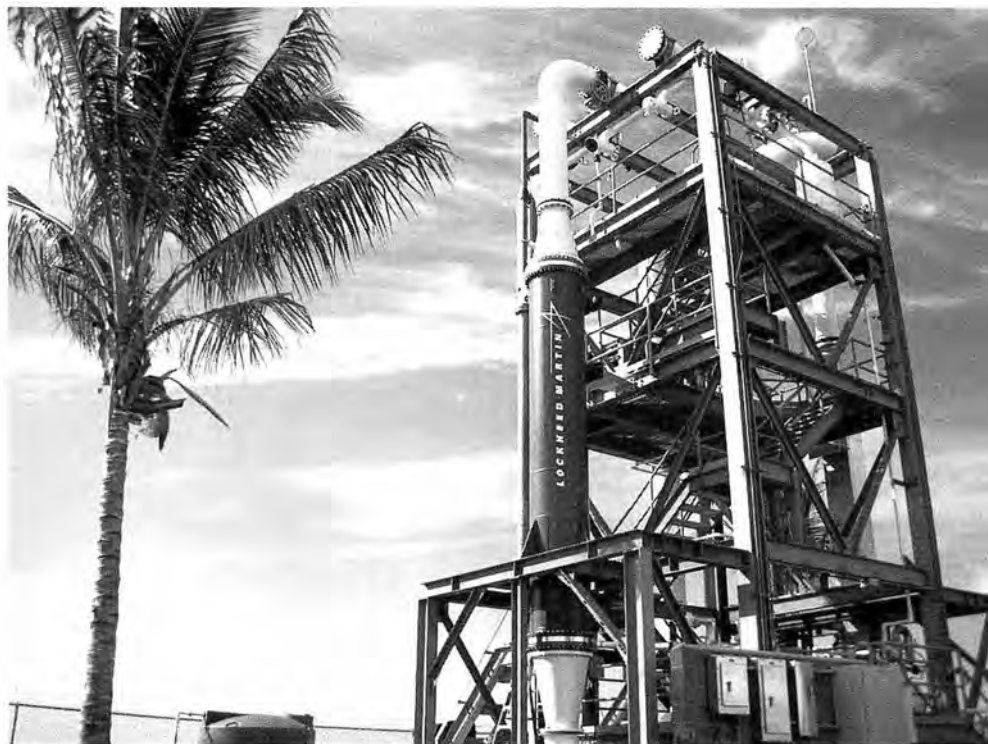
Fig. 2. The Navy funded heat exchange test tower was completed in 2011 and uses anhydrous ammonia as the working fluid. Up to 4 different heat exchangers can be tested and a possible 100 kw turbine is expected to be installed in the future, pending funding.
